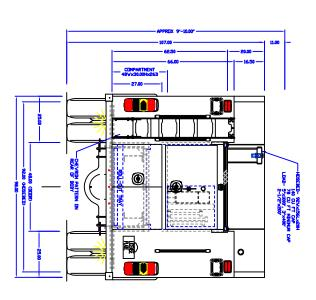
6. THE EFFECTIVE DOOR OPENINGS WILL BE APPROX. 2" LESS THAN THE NOTED COMPARTMENT OPENING FOR ROLL UP DOORS AND UP TO APPROX. 4" LESS FOR HINGED DOORS
